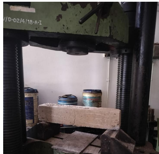
Fig - 1: Flexural Strength Testing
