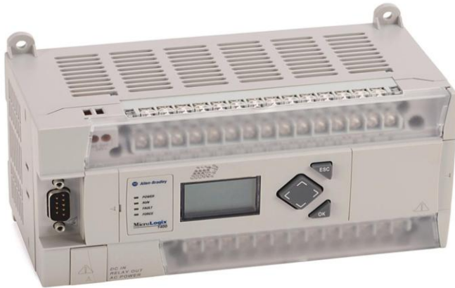
Fig. 5.1. Allen-Bradley MicroLogix 1400 PLC,
