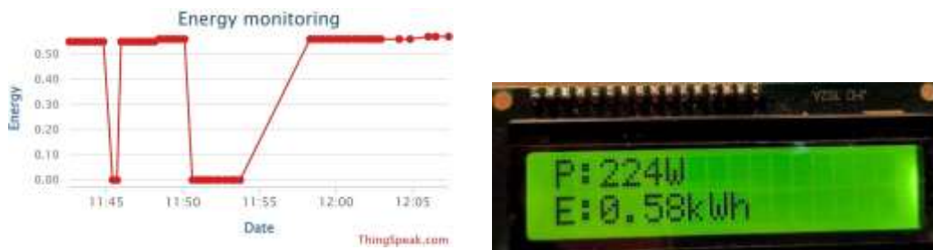
Fig. 4.15: Energy measurement and graph
