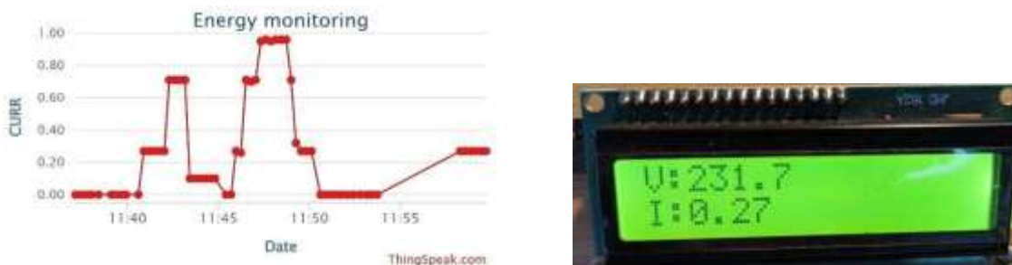
Fig. 4.3: current measurement and graph
