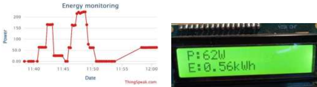
Fig. 4.4 power measurement and graph
