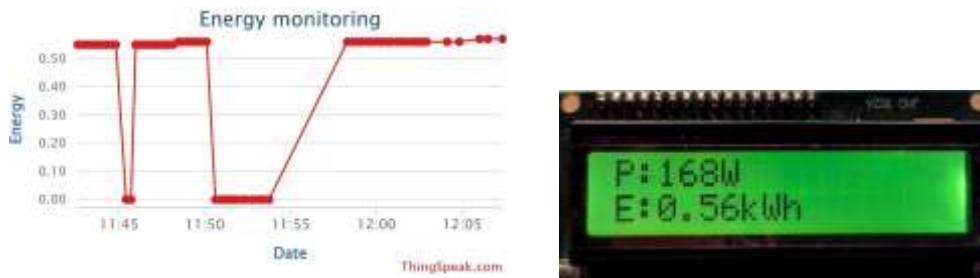
Fig. 4.10: Energy measurement and graph
