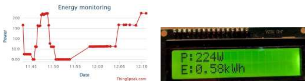
Fig. 4.14: power measurement and graph
