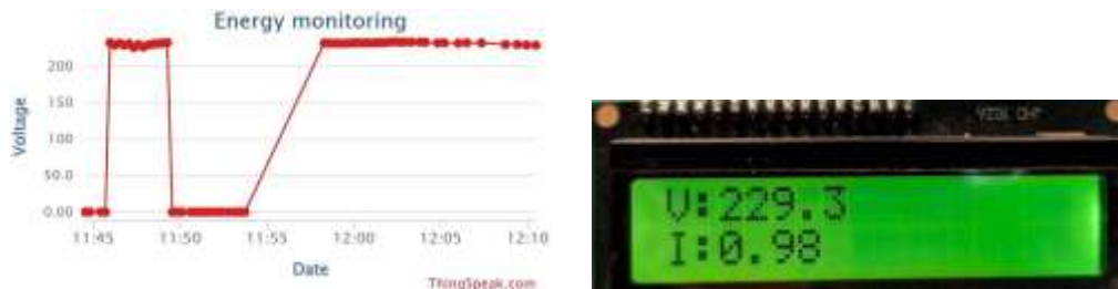
Fig. 4.12: voltage measurement and graph
