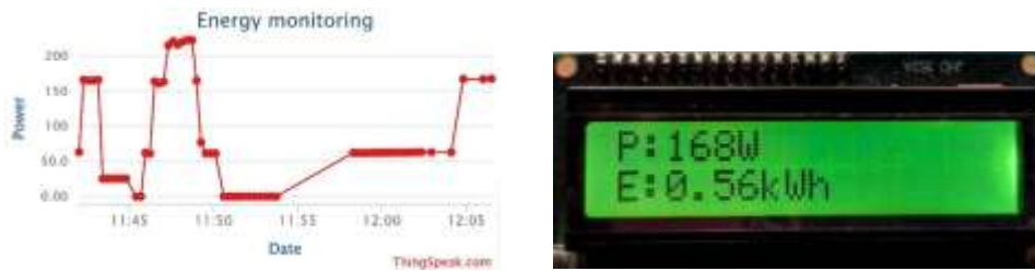
Fig. 4.9: power measurement and graph
