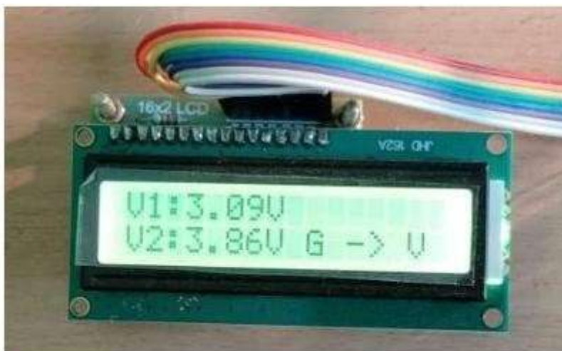
Fig 5.6 LCD Display Showing Solar Voltage, Battery Voltage, and Mode
