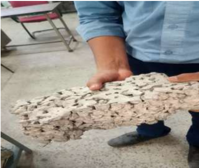
Fig 4: Prototype Pervious concrete block with layers
