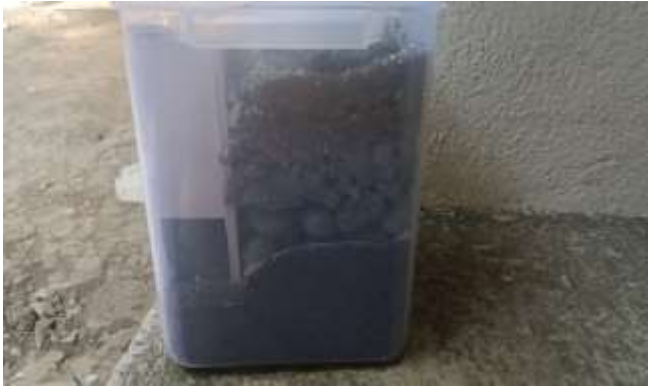
Fig 4: Prototype Pervious concrete block with layers
