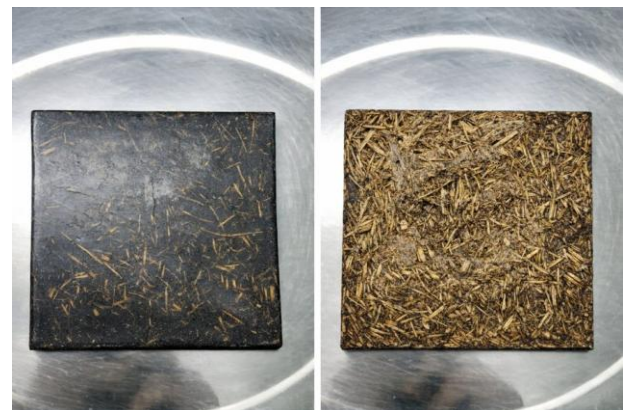
Fig. 2: Fabricated Eco-Panel — smooth front face (left) and textured rear face (right)
