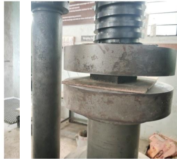
Fig. 4: UTM Compression Test (Result: 1687.5 kN)
