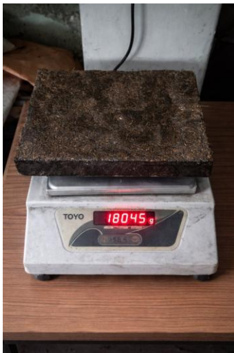
Fig. 5: Panel weight measurement — TOYO digital scale reading 18045 g (18.045 kg)
