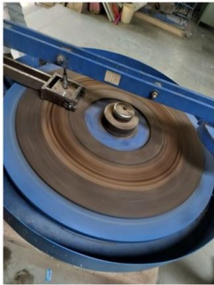
Fig. 3: Abrasion Test (Result: 0.2 mm wear)
