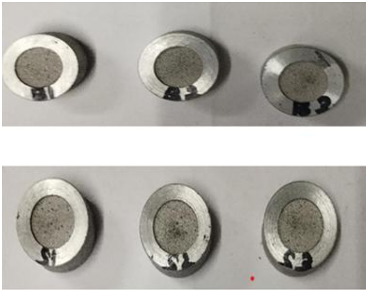
Figure: 5.1 Specimen Image after EDM Process-L16
