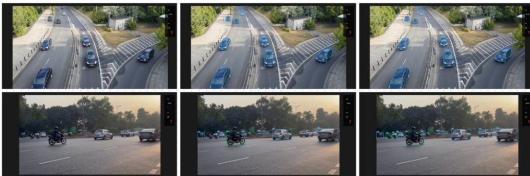
Fig. 5. Qualitative Annotation Results. Each row shows a comparison between the input image (left), AI ensemble predictions (middle), and human-corrected annotations (right). The AI ensemble provides strong initial localisation, significantly reducing manual effort.
