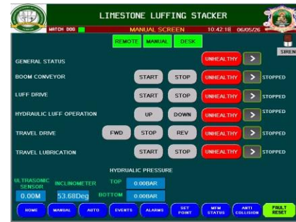
Figure 5. HMI Manual Control Screen
