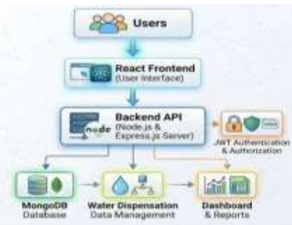
Fig. 2: Smart Water Dispensation System Data Flow
